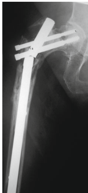
Fig. 25.6 Example of fatigue failure of osteosynthesis. The patient had myeloma affecting the right proximal femur. Intramedullary nail with cement augmentation was used. The patient outlived the implant
